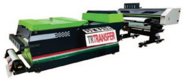
Typical hybrid inkjet print + powder + drying production machine
