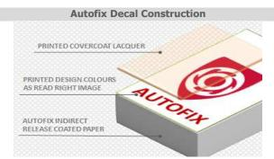
Autofix sheets are screen-printed in controlled RH conditions where the inks are wicket dried using RT air movement only. Inks, precious metals & covercoat lacquers are from specialized suppliers
