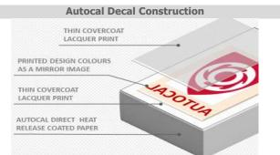
Autocal rolls are web screen-printed where the inks are gently force dried at 40 to 50°C in a festoon dryer using air movement. Inks, precious metals & covercoat lacquers are from specialized suppliers
